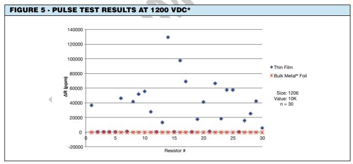
\*Note: Average of 30 units yielded deviation of 30,723 ppm of the thin film vs. -14 ppm for the Bulk Metal® Foil
