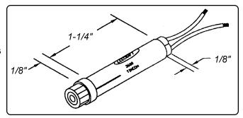
6" Wire Leads Hi-Hat Lens or Flush Lens White Housing Variety of Lens Colors
