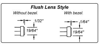
6" Wire Leads Flush Lens White Housing Speed Nut Variety of Lens Colors PressFit
