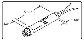
6" Wire Leads Hi-Hat Lens or Flush Lens White Housing Variety of Lens Colors
