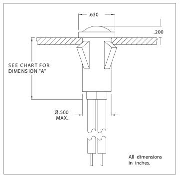
Mounting: Will snap-fit into Ø.500/.505 hole in panels .020/.100 thick. Push-on speednut SN0461 also available. Mounting hole pattern on page SP2.
