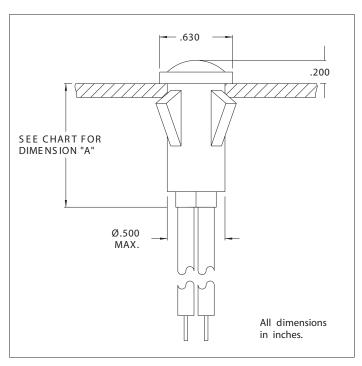
Mounting: Will snap-fit into Ø.500/.505 hole in panels .020/.100 thick. Push-on speednut SN0461 also available. Mounting hole pattern on page SP2.
