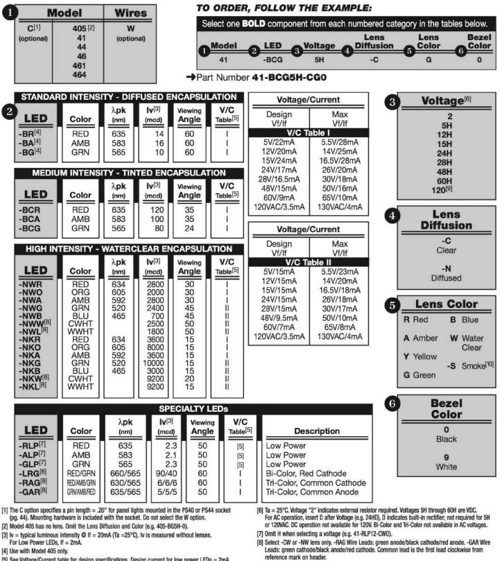
[5] See Voltage/Current table for design specifications. Design current for low power LEDs = 2mA.
