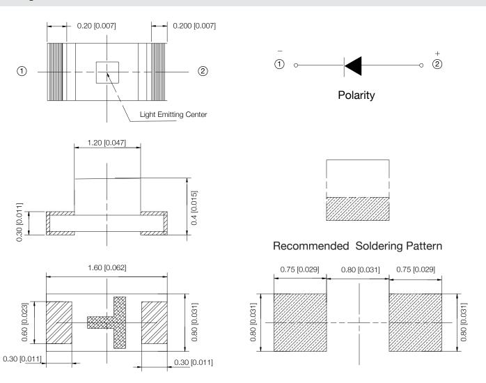
**Note:** The tolerance unless mentioned is  $\pm$  0.1mm [0.005 in]; Unit=mm [in]
