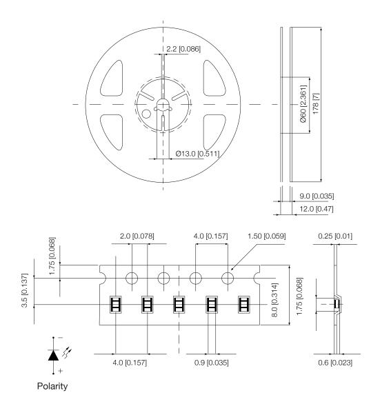
Note: The tolerance unless mentioned is  $\pm$  0.1mm [0.005 in] ; Unit=mm [in]
