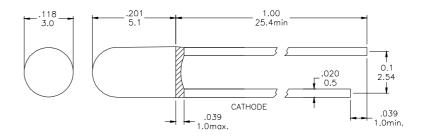
\* Tolerance:  $\frac{0.01}{0.25}$  Unit:  $\frac{\text{inch}}{\text{mm}}$
