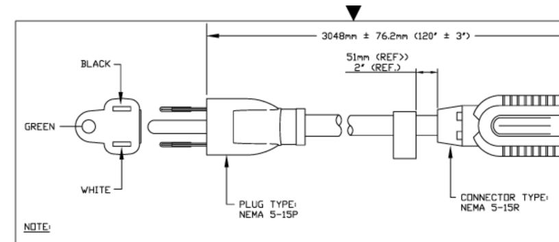
RESTRICTED USE DETACHABLE POWER SUPPLY CORD FOR BUSINESS, MAILING MACHINES AND ELECTRICAL EQUIP. THAT HAVE A BUILT IN RECEPTACLE WITH BLADES AND GROUNDING PIN FOR CORD ATTACHMENT.
