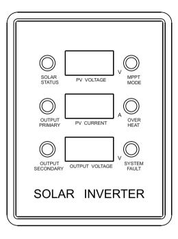
**SOLAR STATUS** - When the PV voltage is greater than 80% of the rated voltage of the device, the indicator lamp will be lit. Otherwise, it will blink. **OUTPUT PRIMARY** - It lights when socket 1 is working **OUTPUT SECONDARY** - It lights when socket 2 is working
