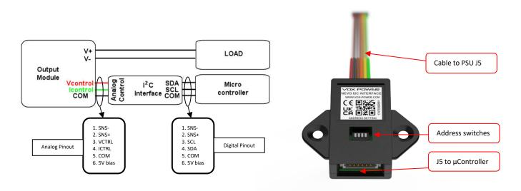
The output voltage and current limit can then be controlled in +/-127 steps that are programmed through the I<sup>2</sup>C interface. Careful consideration must be given to system grounding as the interface is <u>not</u> isolated and must be referenced to the COM pin on J5. Incorrect system grounding may cause damage to the unit. Adhere to the same precautions as for "Local bias supply" detailed on page 16 of the user manual or contact Vox Power for assistance.
