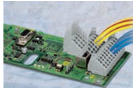
Removing the terminal blocks to place the board
