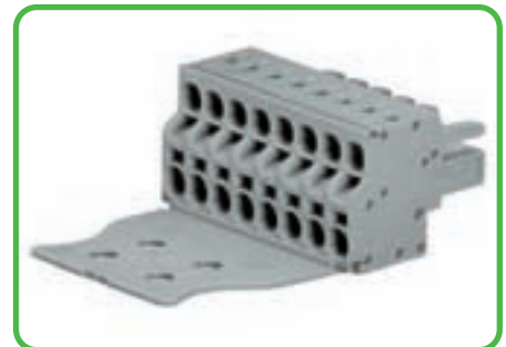
Female connector, pin spacing 5 mm/0.197 in, grey 8 poles, with strain relief plate 231-2108/026-000/135-000
