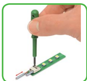
Inserting/removing fine-stranded conductors by lightly pressing on push-button (e.g., using a 233-335 operating tool).
