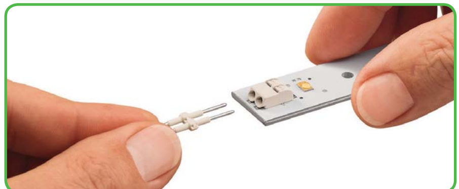
Inserting the connecting link into terminal block.
