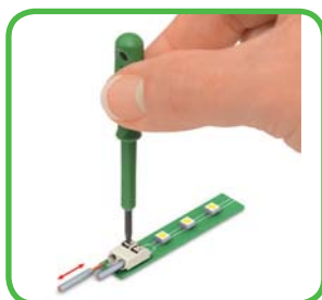
Inserting/removing fine-stranded conductors by lightly pressing on push-button (e.g., using a 233-335 operating tool or a ball point pen).
