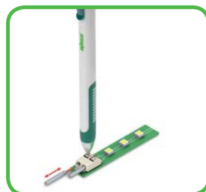
Inserting/removing fine-stranded conductors by lightly pressing on push-button (e.g., using a 233-335 operating tool or a ball point pen).
