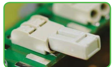
2000-402 Shorting Bar - used to complete the circuit at the end of a string of linear LED modules, e.g., insert with WAGO logo facing upward, and at a slight angle so the bottom of the housing clears the bottom edge of the terminal block wire entry opening.
