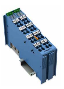
This analog input module directly connects resistance temperature devices (RTD)and thermocouples operating in hazardous environments of Zones 0 and 1. The cold junction compensation of the respective channel is incorporated into the module.
