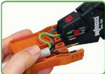
Strip wire ends 9 mm/0.354 in (see marking).
