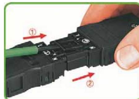
Locking lever, tool operated: 1.) Unlatch locking lever. 2.) Pull apart the connectors. (Example shows 3-pole connector)
