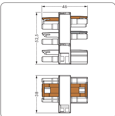
Cable assembly with coding S for connection to 770-637 and 770-638 distribution connectors see page 40.
