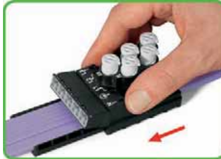
Mount IDC module flush with the bottom part. Should the IDC module jam during mounting, turn the upper part by 180° and remount it.
