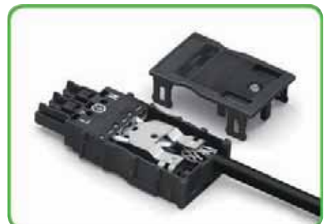
First insert the wired connector into the strain relief housing, then snap the cover and tighten the screw.
