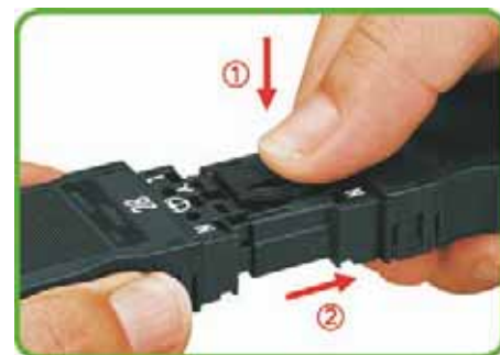
Locking lever, manually operated: 1.) Press on locking lever. 2.) Pull apart the connectors. (Example shows 3-pole connector)
