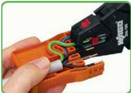
Strip wire ends 9 mm/0.354 in (see marking).
