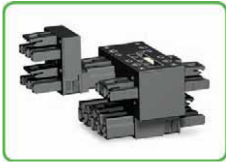
An additional h-distribution connector doubles L1. This results in the following connection options: L1/L1/L2/L2/L3 with jumper in position L2 L1/L1/L2/L3/L3 with jumper in position L3
