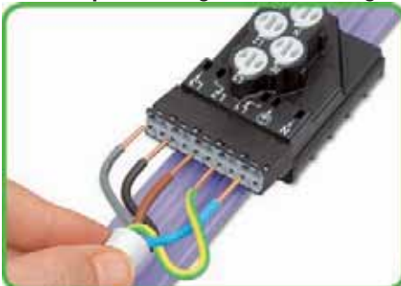
Connecting an installation cable to the supply module. Stripped solid wires can be connected by simply pushing them in. When using stripped fine-stranded wires, open clamping unit using a screwdriver.
