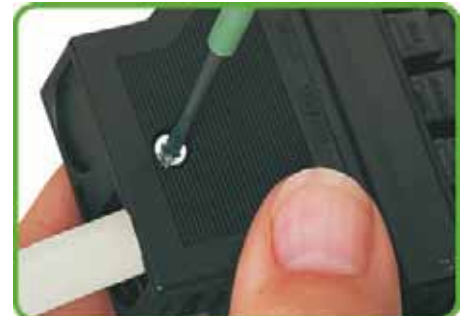
Tighten the strain relief screw using a screwdriver
