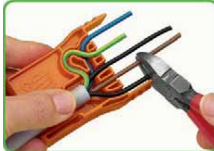
Cut wire ends.
