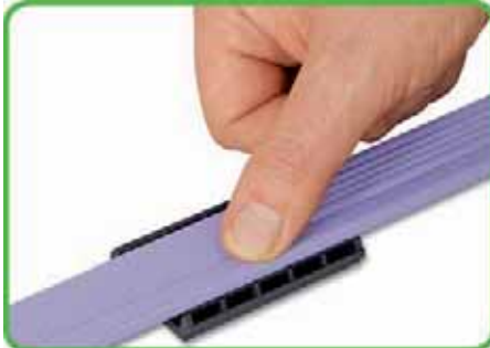
Insert flat cable into bottom part (observe coding!).
