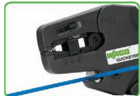
Cutting the conductor.
