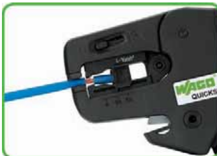
Stripping the conductor.
