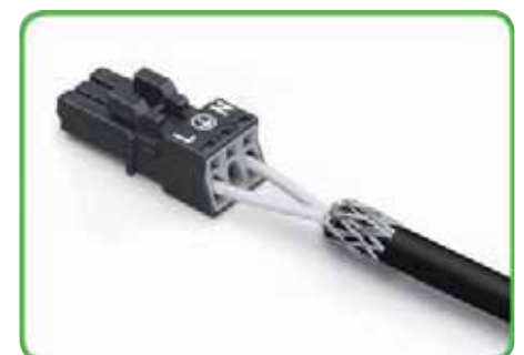
Apply the shield to the rubber cable. Strip length, outer insulation = 30 mm / 1.18 in Shield length = 8 mm / 0.31 in
