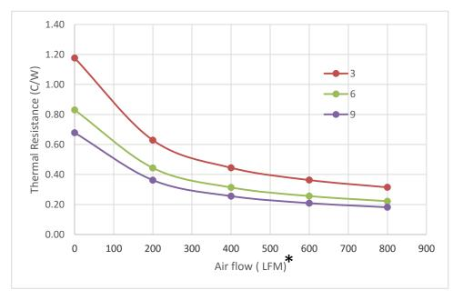
\*Thermal performance data is for reference only and may vary by application \*0 LFM represents a natural convection environment with a vertical heatsink \*All data is based on a fully distributed load on the base of the heatsink \*All forced convection data is based on an open duct configuration
