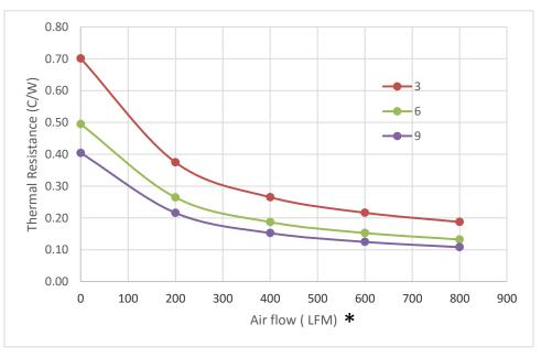
\*Thermal performance data is for reference only and may vary by application \*0 LFM represents a natural convection environment with a vertical heatsink \*All data is based on a fully distributed load on the base of the heatsink \*All forced convection data is based on an open duct configuration
