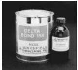
DeltaBond<sup>™</sup> 154 is a medium viscosity, aluminum-filled resin with the best thermal conductivity of this series. It is, however, neither a good electrical insulator nor conductor. Its principal application is that of a good thermal mechanical adhesive for applications such as bonding fins to base plates or structural mounting blocks or brackets to heat sinks. Shelf life: 2 years.
