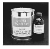
**DeltaBond™** 154 is a medium viscosity, aluminum-filled resin with the best thermal conductivity of this series. It is, however, neither a good electrical insulator nor conductor. Its principal application is that of a good thermal mechanical adhesive for applications such as bonding fins to base plates or structural mounting blocks or brackets to heat sinks. Order one bottle of hardener A4 or B4 per one quart of **DeltaBond™** 154 separately. Shelf life: 2 years.
