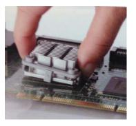
STEP 1: Center heat Sink onto BGA. Tilt and hook one side of the clip under the BGA chip.
