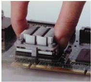
STEP 2: Press down the other side of clip to snap it onto the BGA chip.
