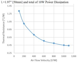
NOTE: Natural Convection Thermal resistance 2.10 °C/W based on 70 °C Temp rise about ambient.
