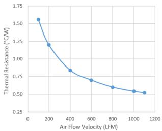
NOTE: Natural Convection Thermal resistance 2.50 °C/W based on 70 °C Temp rise about ambient.
