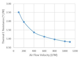
NOTE: Natural Convection Thermal resistance 4.06 °C/W based on 70 °C Temp rise about ambient.
