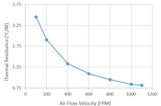
NOTE: Natural Convection Thermal resistance 3.94 °C/W based on 70 °C Temp rise about ambient.
