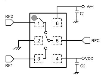
Note: No DC Blocking capacitors are required because of the all RF ports integrated DC blocking capacitors.
