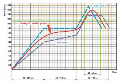
Fig 2. Infrared soldering profile
