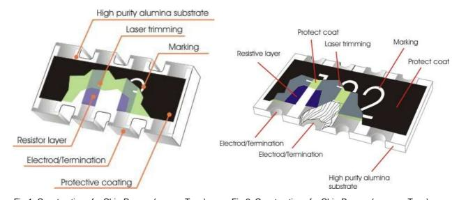
Fig 1. Construction of a Chip-R array (convex Type)
