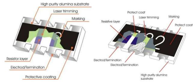
Fig 1. Consctruction of a Chip-R array (convex Type)
