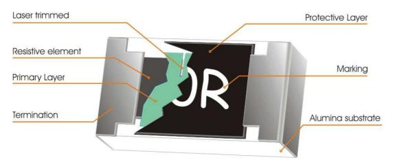
Fig 1. Construction of Chip-R
