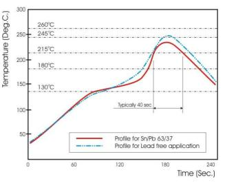
Fig 3. Infrared soldering profile for Chip Resistors
