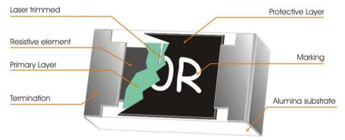
Fig 1. Construction of 2512, 2010 Chip-R
