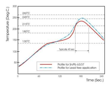
Fig 4. Infrared soldering profile for Chip Resistors
