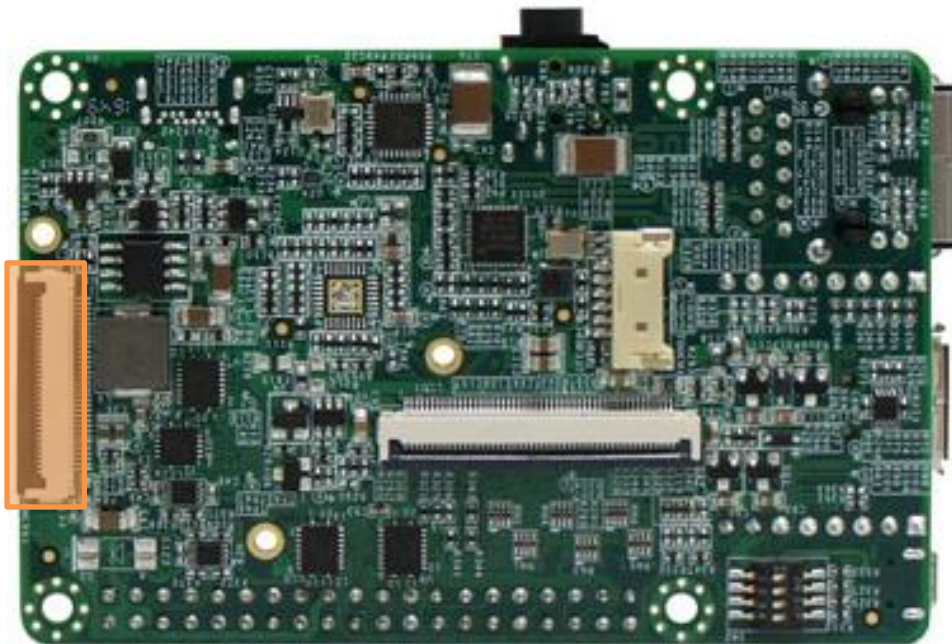
Figure 24 - PICO-PI-IMX7 Touch Panel Connector Location
