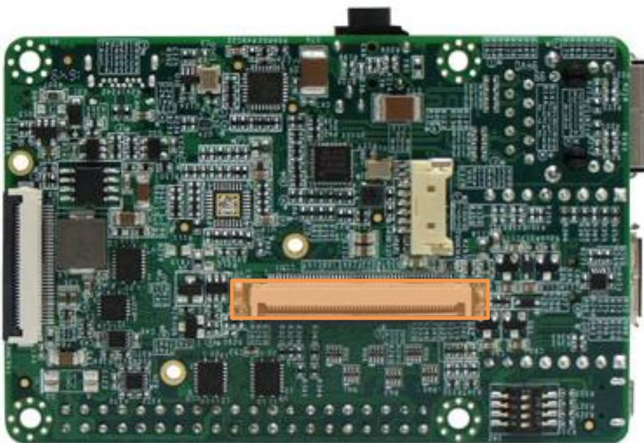
Figure 22 - PICO-PI-IMX7 LCD Display FPC Connector Location
