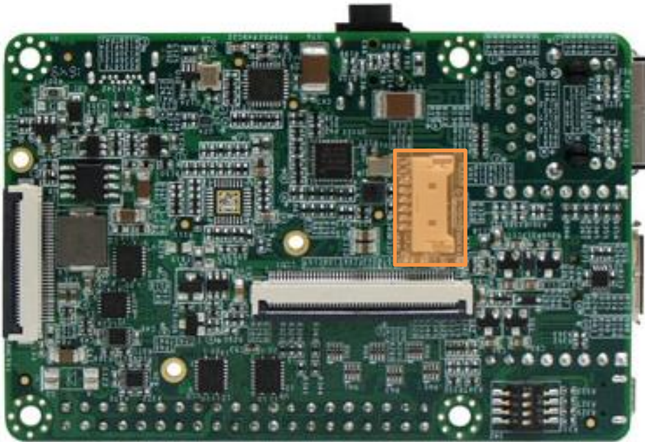
Figure 23 - PICO-PI-IMX7 Touch Panel Connector Location
