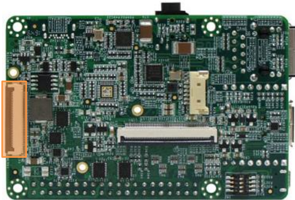
Figure 24 - PICO-PI-IMX7 Touch Panel Connector Location
