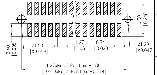
Recommended P.C.B Layout (Top Side) (PCB BOARD TOLERANCE ± 0.05)
