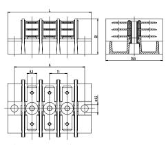
L = (Number of poles x Pitch) + 19,3 A = (Number of poles + 1) x Pitch Shown type of tab connector package: 5.033
