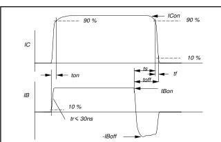
Fig.4. Switching times waveforms with resistive load.
