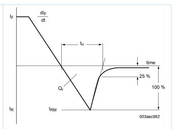
Fig. 7. Reverse recovery definitions; ramp recovery
