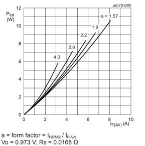
Vo = 0.973 V; Rs = 0.0168  $\Omega$ Fig. 2. Forward power dissipation as a function of average forward current; sinusoidal waveform; maximum values
