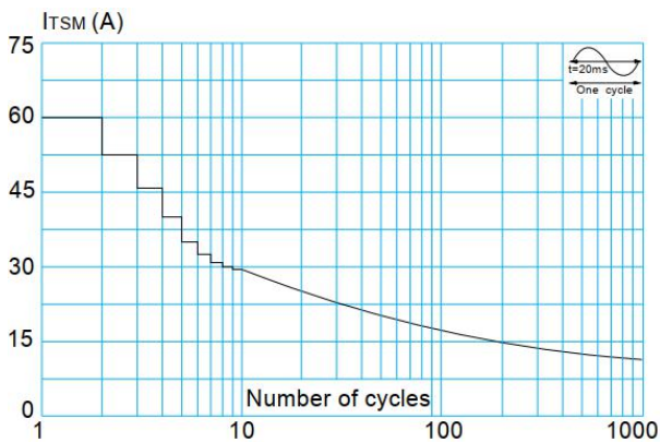
FIG.5: Non-repetitive surge peak on-state current for a sinusoidal pulse with width t_p < 20\text{ms} , and corresponding value of I^2t ( I - II - III: di/dt < 50\text{A}/\mu\text{s}; IV: di/dt < 10\text{A}/\mu\text{s} )
