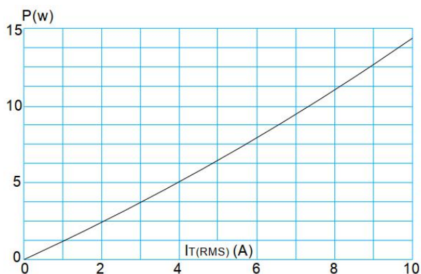
FIG.1: Maximum power dissipation versus RMS on-state current
