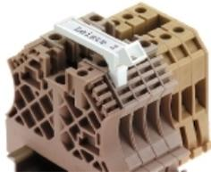
The SchT 5 S group tag carriers are clipped directly onto the TS 32 mounting rail (G-rail) or the TS 35 mounting rail (top-hat rail). It is therefore possible to label the terminal strip irrespective of the terminal and the type of terminal. SchT 5 and SchT 5 S are fitted with ESO 5, STR 5 protective strips.
