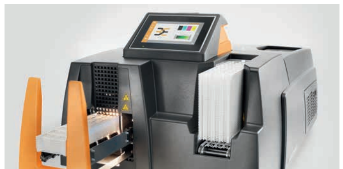
High magazine capacity for loading and dispensing of up to 50 MultiCards.
