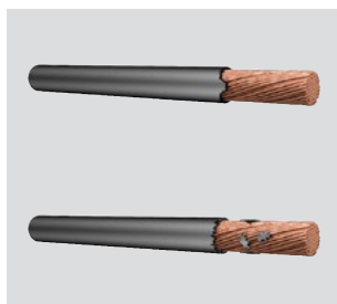
Insulation has not been cut properly
