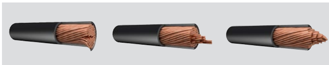
Conductor sheared off Conductor pulled out Squeezed cable
