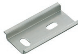
TS 35/7.5 mm according to EN 50022 (s = 1.0 mm)
