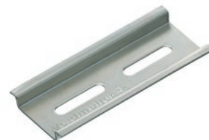
TS 15/5.5 mm according to EN 50045 (s = 1.0 mm)
