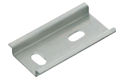
TS 35/7.5 mm according to EN 50022 (s = 1.0 mm)
