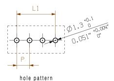
For the mounting of PCBs, it should be noted that the rated data given in the catalogue relates only to the connection elements. The neccessary creepage and clearance paths must be observed in connection with the respective applicant in accordance to VDE 0110. The current-carrying capacity and pitch tolerance is to be determined according to DIN IEC 326 part 3 very fine.
