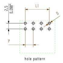
For the mounting of PCBs, it should be note rated data given in the catalogue relates on connection elements. The neccessary creep clearance paths must be observed in connet the respective applicant in accordance to V The current-carrying capacity and pitch tole be determined according to DIN IEC 326 pa
